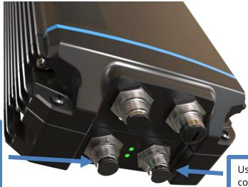
The power connector is on the left-hand side when the logo is facing up.
