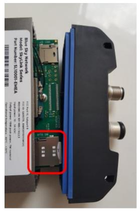
**NOTE**: A micro SD slot is also present behind the connectivity port. Ensure that the SIM cards are placed into the correct holders and not the micro SD slot. If the device does not work after installing the SIM cards, they may be in the wrong slots.
