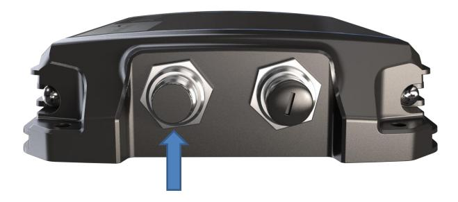
To power on the device, remove the connector cap from the power port located on the bottom panel of the unit. Connect the power cable into the port and the adapter into the appropriate power source (e.g., a wall or vehicle outlet).
