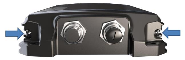
2. Insert SIM cards located behind the connectivity port, taking care to ensure wires remain tucked in.
