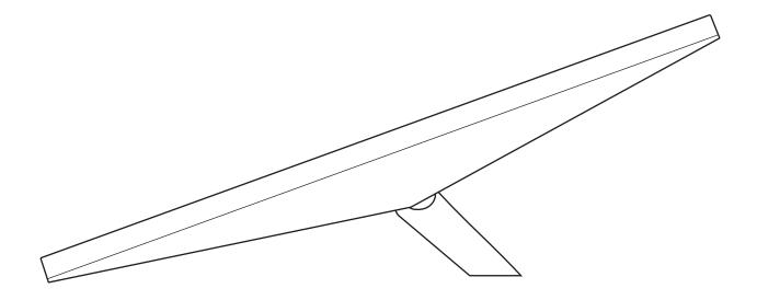
The Starlink Mini Wall Mount is designed for installation on an exterior wall near the top of the gable or fascia. This wall mount can accommodate a 4" overhang maximum and offers a secure, long-reaching platform to optimize the placement of your Starlink for the best connectivity and performance.
