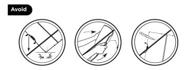
Behaviors above that demage the solar panel, will cause the cell inside the solar panel to crack and efficiency drop, or even unusable. The free warranty period does not cover damage resulting from improper use of the product.
