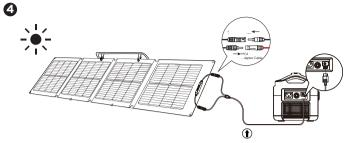
This cable can only be used for connection between solar panels and energy storage. It is prohibited to be used for interconnection between solar panels or other connection purposes.
