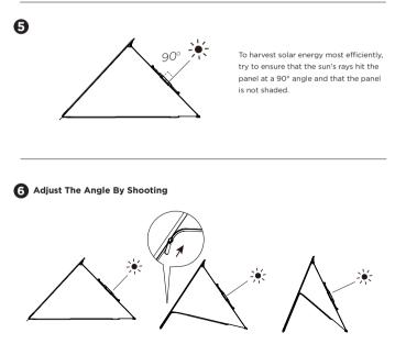
For improved charging results, the Protective Case can also be used as a kickstand to prop up the solar panel at a 25°-80° angle.
