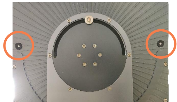
Figure 4 Protective vents on backside of antenna.
