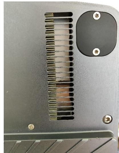
Figure 3 Air exhaust at the backside of antenna.
