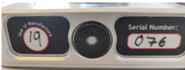
Figure 5 Protective vent on base part of terminal next to the Serial Number.
