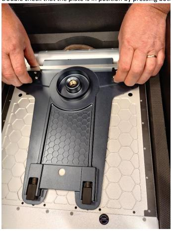
Lift up and turn the Terminal and place the round part of the plate onto the center of the tripod.
