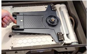
Press both hooks at the same time and make sure the plate gets into position.
