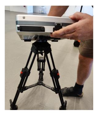
With the terminal resting on the tripod, Hold the side that is furthest away from the center with one hand, and use the other hand to screw the handle placed underneath the tripod.
