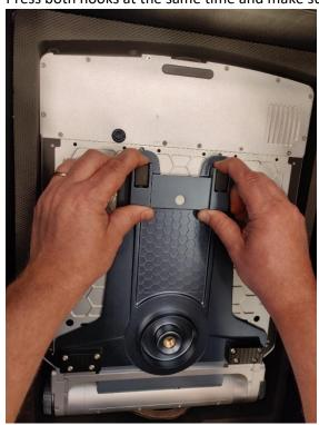
Double check that the plate is in position by pressing both sides
