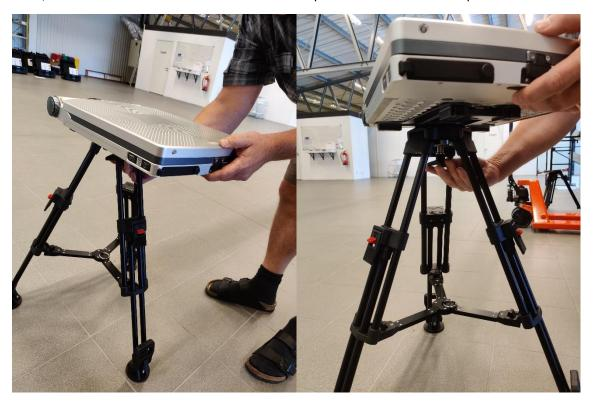
Screw it all the way in, and then make sure the terminal is in position.
