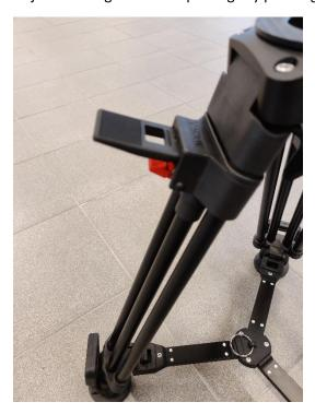
Place the tripod in a suitable position and height and use the libel to make sure the tripod is leveled. Detach the spreaders if needed.
