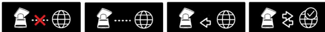
Figure 17 Connection to modem not working in the left picture, connection established to modem in the middle-left picture, terminal receive lock in the middle-right picture, terminal also transmitting with an established internet connection to the right.
