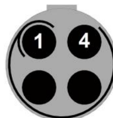
Figure C2 DC connector pin layout (terminal view).
