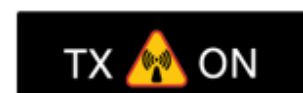
Figure 20 Terminal transmit is turned on and led on top of antenna is on. Warning: See the safety instructions for operating terminal.
