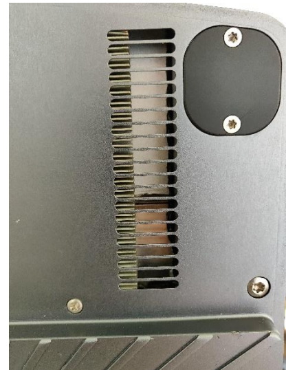
Figure 32 Air exhaust at the backside of antenna.
