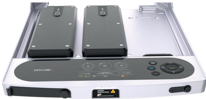
Figure 7 Connection ports are located on the front of the terminal. The DC power cable socket is located to the right. Ethernet and USB ports are located to the left. Left ethernet port is labeled LAN 1 and the right LAN 2.
