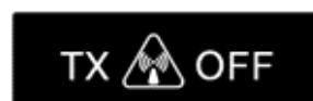
Figure 19 Transmission has been approved by user, pointing or other criteria for transmission not yet fulfilled.
