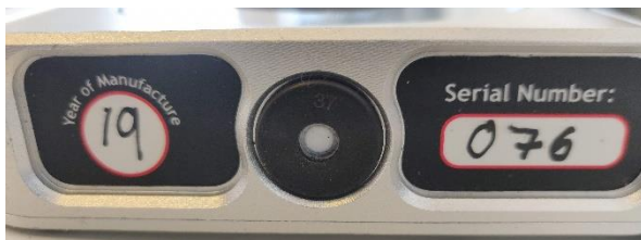
Figure 34 Protective vent on base part of terminal next to the Serial Number.
