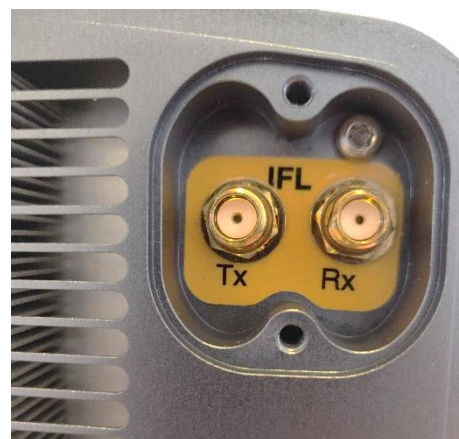
Figure C3b L-band interface, 50 ohms SMA connectors exposed.
